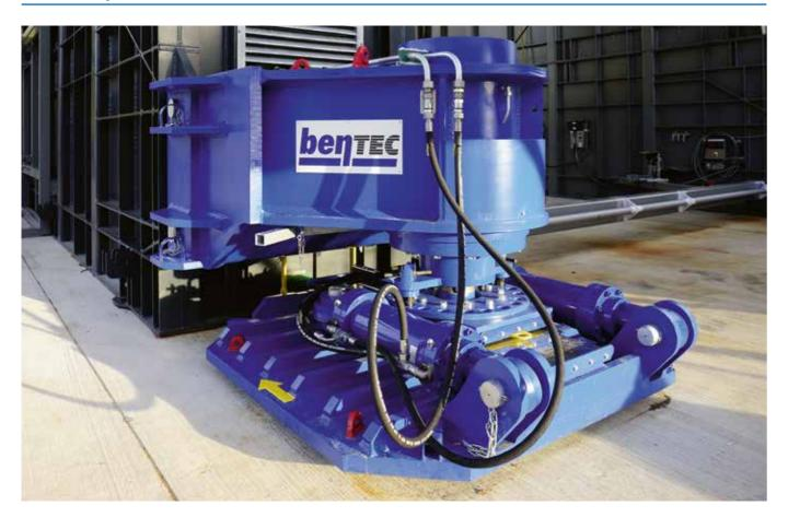
Bentec Rig Walking Systems provides a solution for reducing the time taken for a rig move on multi-well rig-sites. Moving the complete rig to the next well also requires fewer cranes and less manpower.
